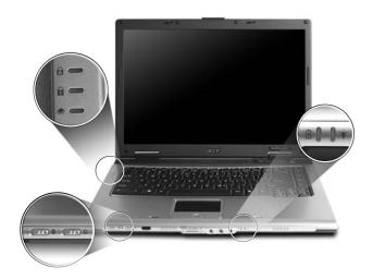
The power, battery and wireless communication status indicators are visible even when the LCD display is closed.
